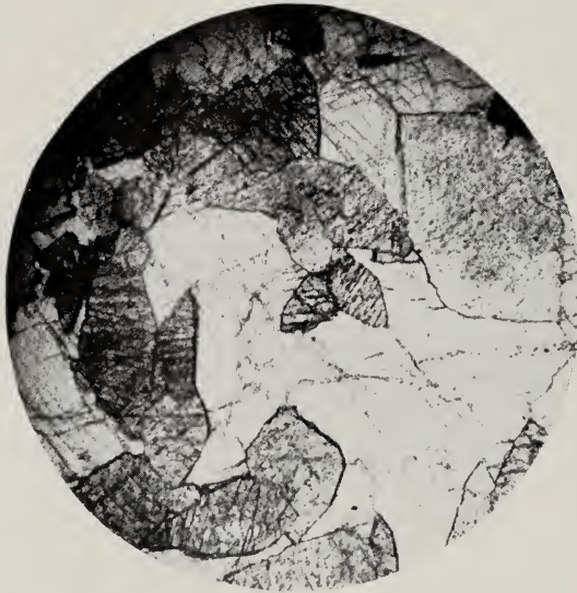
FIG. 25. Photomicrograph of fine inter-growth of calcite (dark) and fluorite (light) from the Hillside vein. Note the crystal outlines of the calcite, which show that it had not been replaced by fluorite.
